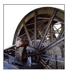
New chances of silver mining occurred after the invention and the setup of steam engines in the 19th century. Even in 1750 mining was in progress only with some simple tools, in depths around 100 m. The expansion came in 1879 with the usage of a steam engine with very high performance, when for the first time in the world depth of 1 km was broken. This record was not broken for a long time.
